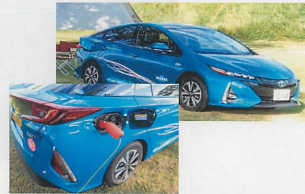
The external power supply of a PHV
